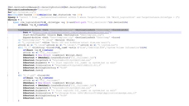
Backdoor sends system information and IP address (using ip-api) to C2 Server.
